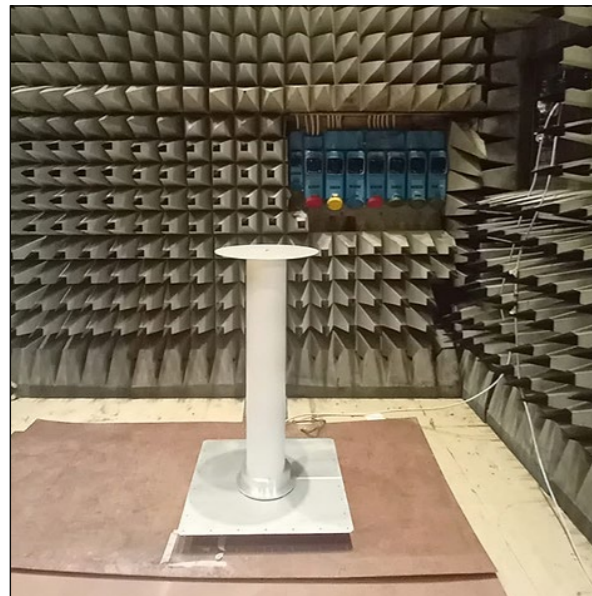
(l) antenna in the anechoic chambers for the test measurements (courtesy of Free Space S.r.l.)
