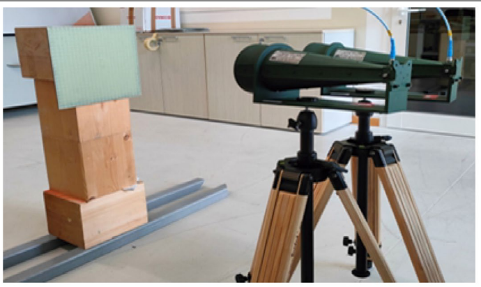
(b) Measurement of the reflection coefficient of a passive metasurface panel
