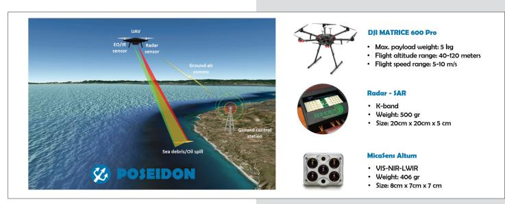
(a) - POSEIDON system and its main components
